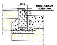
**DETALLE "B" BORDILLO DE CONFINAMIENTO SIN ESCALA**
